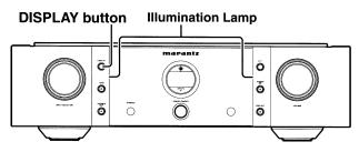
The illumination lamp has an always-ON mode (factory setting) and an always-OFF mode.
